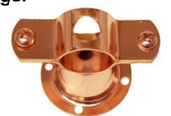
Our Copper Plated Bell Hanger has a patented access hole through the top which allows the hanger to be mounted to most flat surfaces without disassembling the cap. We have added 4 additional mounting holes around the base of the bell for additional mounting flexibility. Our hanger is used as a standoff clamp in both vertical and horizontal applications and provides 3/4" standoff.
